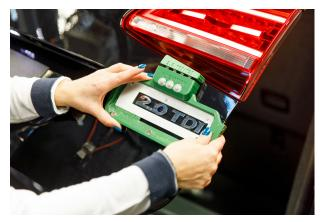
No tooling or machining is required to build a model. The cost is far less than traditional manufacturing methods, and the results can be tailored to match exact requirements.
